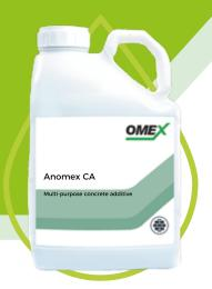
ANOMEX CA is a calcium nitrate solution developed for the construction industry as a multi-purpose concrete admixture which is used as a concrete setting accelerator even in cold temperatures. Calcium increases the rate of early hydration of the concrete, thus, a speedier setting time and strength development of the concrete is achieved.
